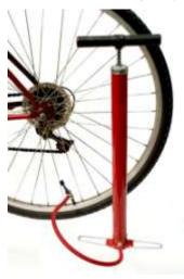
A flat tire is not very useful. It does not cushion the rim of the wheel and creates a very uncomfortable ride. When air is added to the tire, the pressure increases as more molecules of gas are forced into the rigid tire. How much air should be put into a tire depends on the pressure rating for that tire. Too little pressure and the tire will not hold its shape. Too much pressure and the tire could burst.
