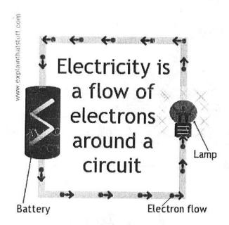
Electricity can move around a circuit in two different ways. In the big picture up above, you can see electrons racing around a loop like race cars on a track, always going in the same direction. This type of electricity is called **direct current** (DC) and most toys and small gadgets have circuits that work this way.
